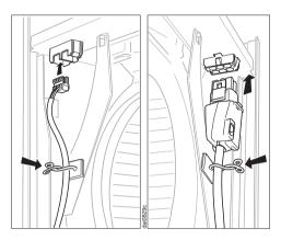
Plug the 2 connectors on the canopy into the corresponding receptacles left and right of the motor assembly.
